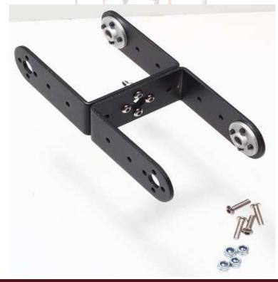
**Step 7:** Now take both assembled structures as shown below along with 2 x M3 Mid Screws, 2 x Nuts and 2 x Bearings.
