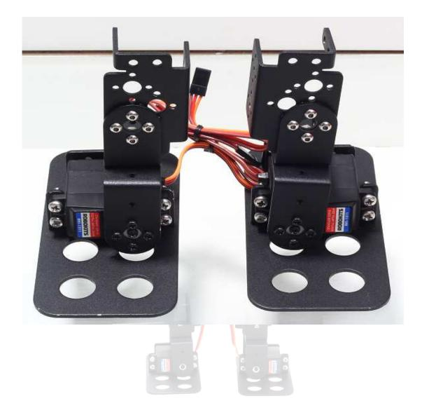
Step 6: Now take 2 x Long U Brackets, 2 x Servo Horns and 8 x Servo Screws as shown below.
