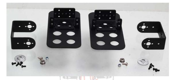
Fix the Servo Horns with the help of Servo Screws on the Short U Brackets. This Short U Brackets will be fixed to the Robot feets with the help of M3 Mid Screws, Nuts and Bearings. Below image shows how it looks after fixing.
