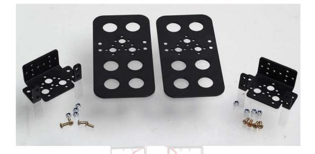
Fix the Multipurpose Brackets on the Robot Feets with the help of CSK Screws and Lock Nuts. The assembly will look as shown in the below Image.
