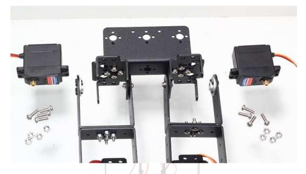
Fix both the Servos at Place 1 and 2 as shown below. Also neutralize the Servo Motors and tight the Servo Screws on the Shaft of Motor once Neutralized.
